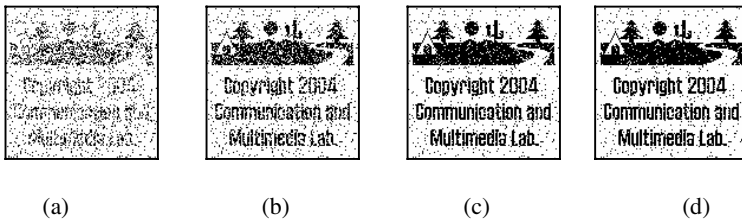
Fig. 7. Extracted watermark patterns after performing (a) 1 generations, (b) 100 generations, (c) 10,000 generations and (d) 1,000,000 generations of optimization computations, given that the pre-specified PSNR requirement is 36dB, are listed for visual evaluation
