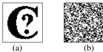
Fig. 9. (a) The extracted logo image from the watermarked Venus model, (b) The extracted logo image from the unwatermarked model
